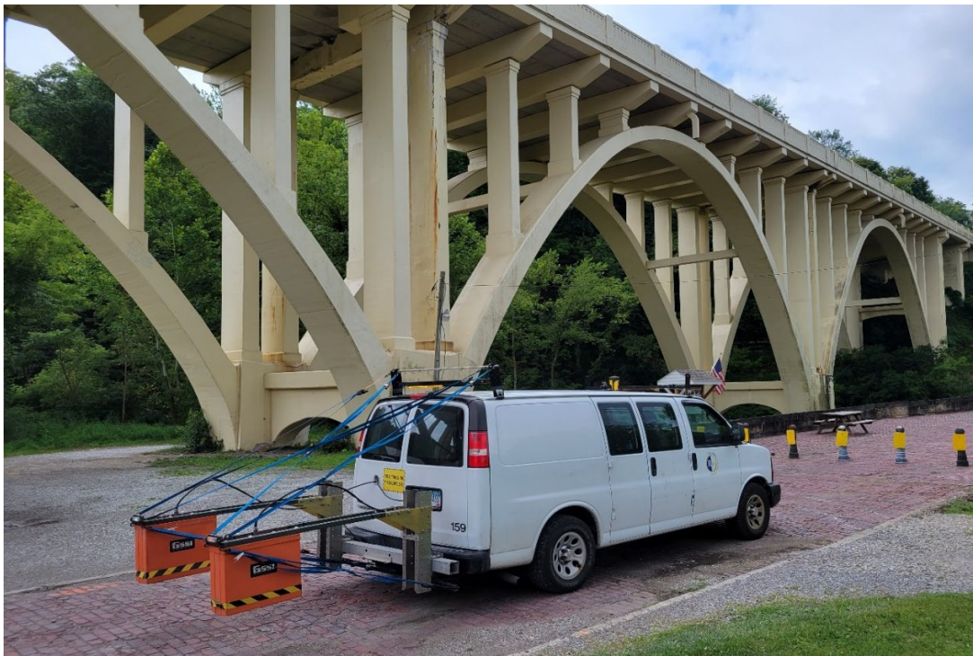
Figure 1. Rii's van-mounted GPR air-launched antennae survey vehicle
