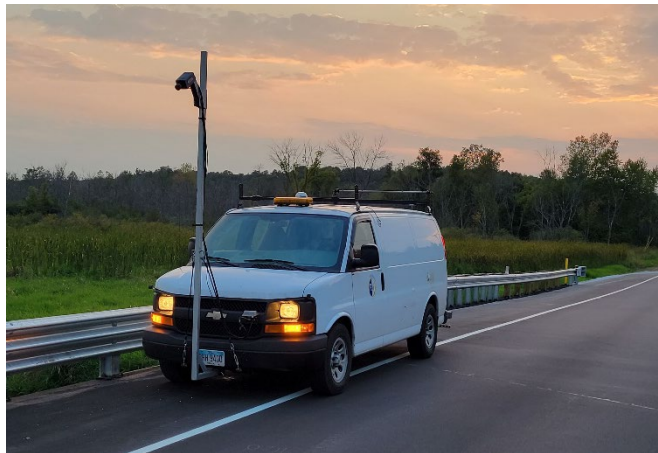
Figure 2. Infrared thermography bridge deck survey vehicle
